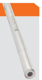
The use of corrosion resistant Hastelloy C-276, gold, and sapphire as the only wetted materials allow the Process BallProbe to withstand the harshest chemical environments. The Process BallProbe was inserted in 350°C hydrothermal vents at the bottom of the Pacific Ocean to obtain Raman data for the monitoring of biomass conversion in supercritical fluids.
